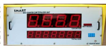
The instrument is Microcontroller based, SWITCH MODE POWER SUPPLY UNIT (SMPS), KEYPAD for programming & counter setting & resetting, seven segment display unit for displaying running COUNT, TOTALISER, SET/PRESET COUNT/TRUCK / WAGON NO. Use of Diffused Optical sensors gives good results, longer life in dusty (CEMENT INDUSTRY) and rough industrial atmosphere.
